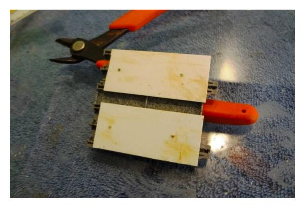
Photo 2 shows the underside of the track. I cut two .08" styrene strips to 25mmX60mm (1"x 2 3/8") and aligned them to be flush with the temporary styrene shim.
