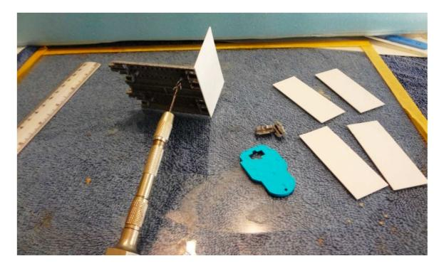
Photo 1 shows a piece of the double concrete Unitrack *with unijoiners removed* and the bolsters being bored out. A 1mm (.04") styrene shim has been temporarily "glued" to the face of the Unijoiner to establish the correct offset for the styrene strips which will be attached to the underside.
